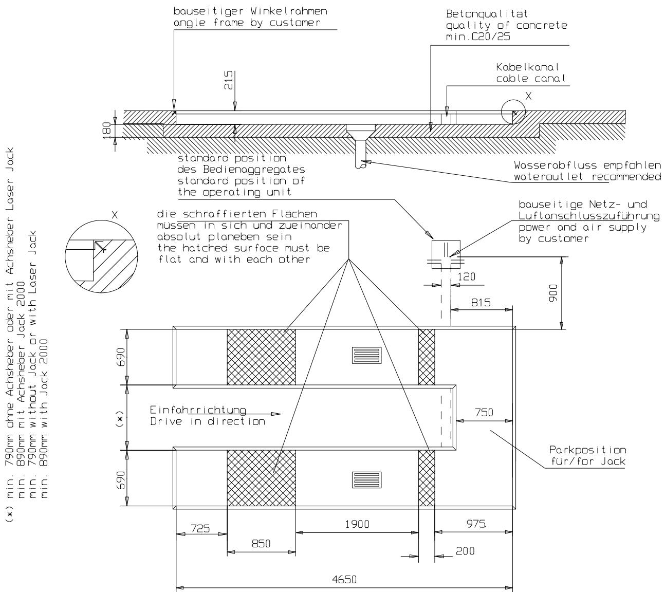
Valid for standard inground version of the lift with drive-on ramp at each side of the platform.
