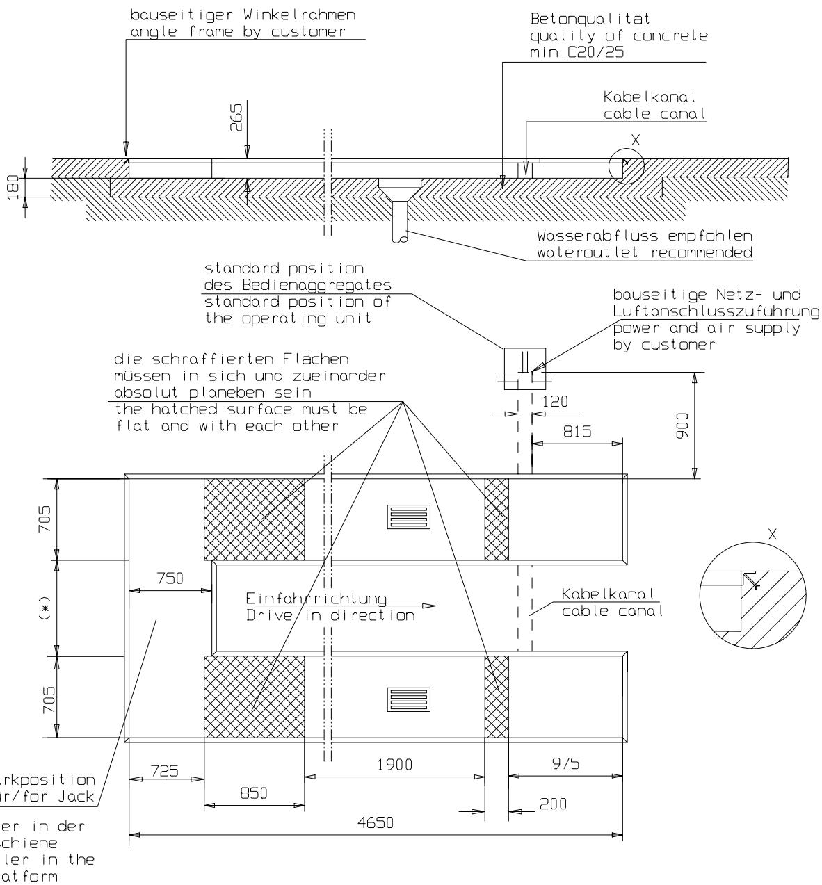
Valid for standard inground version of the lift with drive-on ramp at each side of the platform.
